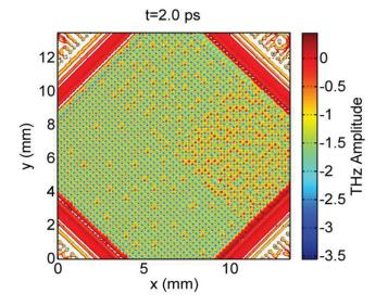
Example plots of the THz near-field distribution measured at a metamaterial surface for sensing applications which is locally loaded with sample material. Left: Peak excitation state, right: 2 ps after excitation.
