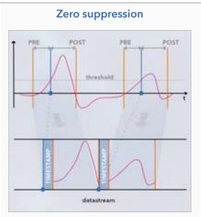
Detect pulses above a certain threshold and only acquire the relevant data to massively reduce the amount of data that needs to be copied and analysed. Configurable DC Offset
