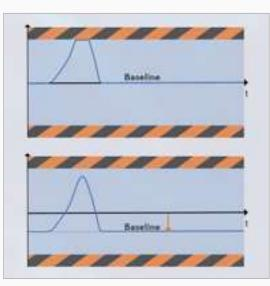
When acquiring unipolar pulses, shift the baseline to the edge of the ADC range to double your dynamic range compared with conventional ADC boards.
