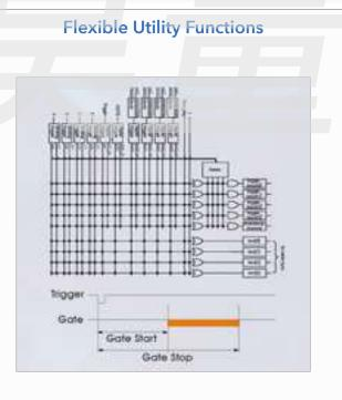
A multitude of useful details help you to create a highly integrated setup with a minimum of external components. Using the integrated TiGer timing pattern generator can provide digital pulse patterns to control your experiment or internal triggers. Use gate and veto functions with our gating logic. This also works across channels or from the additional digital input with a flexible trigger matrix.
