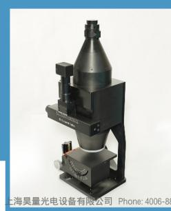
Measure the scattering from a sample in realtime, at high resolution, and with great ease of use.
