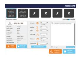
**PC control software -** For system integrators ML6600 is available as a subsystem which can be directly controlled with digital control signals through RS422, RS232 or Ethernet. Analog trigger signals are optionally available. ML6600 can also act as a stand-alone version, which comes with a PC software with elegant graphic UI.
