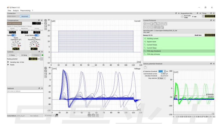
Snapshot of the EZ patch interface demo mode during the application of a series of current-steps to the single cell FitzHugh-Nagumo (FHN) model. The action potential threshold analysis tool automatically calculates both the AP threshold and the sub threshold current values. The analysis can be exported as row data within a .csv file.
