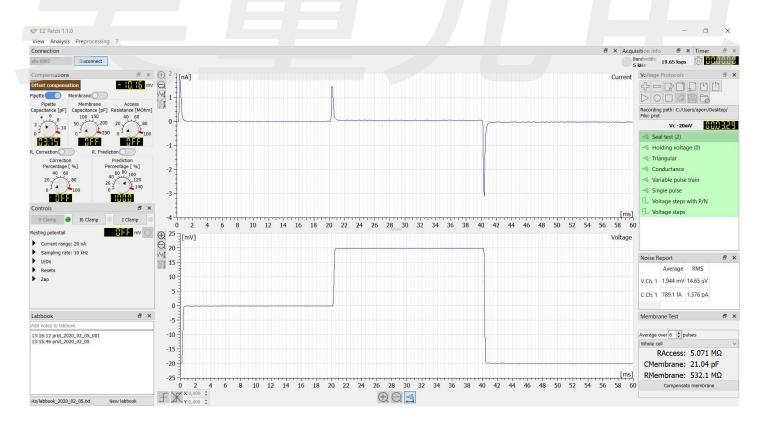
The figure shows the EZ Patch software interface. The oscilloscope window displays a triggered view of a defined continuous square wave applied to monitor the cell parameters. The real time analysis of the current response provides a range of measurements (Cm, Rm and Ra) shown within the membrane test widget (bottom, right of the GUI).
