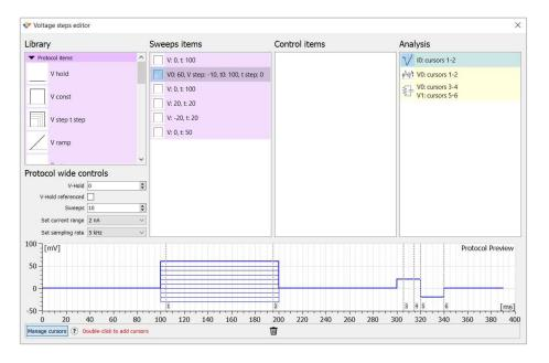
The voltage protocol editor is designed to easily set up all the various aspects of data acquisition, ranging from the acquisition mode, the sampling rate, the gain, the shape of the command waveform and much more...
