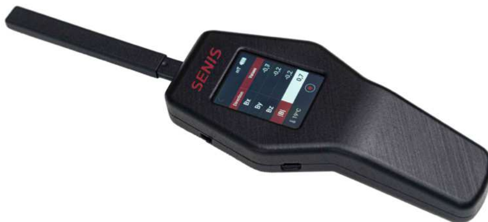
Figure 1: SENIS 3MH1 Handheld Teslameter
