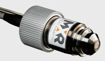
The LightBright is an end window X-ray tube designed for customers that require maximum flux, short FOD and a wide beam angle. The large heat sink directly coupled to the anode provides efficient heat transfer enabling continuous high current operation, and the optimized filament design provides full beam current down to 4kV without sacrificing tube life. The integrated Mammoflex® HV cable and LV cables allow for easy connection to a standard HV power supply.
