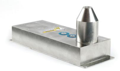
**Model M25:** 50 kV, 4W X-ray Monoblock - The M25 x-ray monoblock is a fully integrated miniature 50 kV, 4W x-ray generator designed specifically to be used as component of a handheld, portable, or bench top x-ray instrument. The source includes a miniature sealed x-ray tube with a transmission-type end window, a high voltage power supply, and control electronics contained in a compact grounded enclosure.
