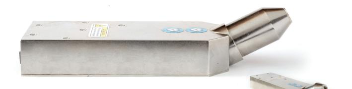
**Model M54:** 50 kV, 4W X-ray Monoblock - The M54 x-ray monoblock is a fully integrated miniature 50 kV, 4W x-ray generator designed specifically to be used as component of a handheld, portable, or benchtop x-ray instrument. The source includes a miniature sealed x-ray tube with a transmission-type end window, a high voltage power supply, and control electronics contained in a compact grounded enclosure.
