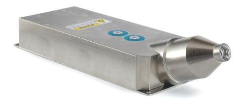
**Model M47:** 50 kV, 10W X-ray Monoblock - The M47 x-ray monoblock is a fully integrated miniature 50 kV, 10 W x-ray generator designed specifically to be used as component of a handheld, portable, or benchtop x-ray instrument. The source includes a miniature sealed x-ray tube with a transmission-type end window, a high voltage power supply, and control electronics contained in a compact grounded enclosure.
