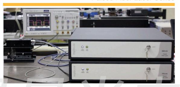
MPBC's line of Nanosecond and Sub-Nanosecond Pulsed Fiber Lasers deliver optimal flexibility for application refinement. Controlled by our straightforward GUI interface, user-selectable parameters include power, repetition rate, pulse time delay and triggering mode - putting more options into the hands of the user.
