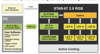
in parallel, conveniently controlled from the same application program and precisely synchronized by the trigger facility. The ALP-4.2 API is well proven and the DLL supports C++, C#, Visual Basic (.NET), Python, MATLAB, LabVIEW, and other development platforms. Microsoft® operating systems are supported up to the most recent Windows® versions both, 32-bit and 64-bit. The ALP-4 USB 2.0 driver is robust, validated, UIF compliant and 24/7 proven in industrial and medical use.\*
