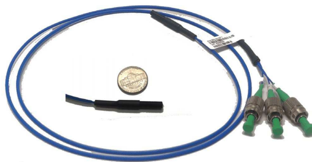
Photos of packaged electro-optic sensor
