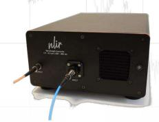
The NLIR U2050 Wavelength Conversion Module converts the mid-infrared wavelengths 1.9 – 5.3  $\mu$ m to the near-infrared wavelengths 682 – 886 nm without any need for alignment. It is just fiber in and fiber out.
