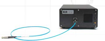
The NLIR MIR Spectrometer is based on a novel measurement scheme that upconverts the MIR light to near-visible light. Silicon-based near-visible light detectors are far superior to MIR light detectors in terms of detectivity, speed and noise. The NLIR upconversion technology therefore brings these attractive features, and the advantages that follow, to the MIR regime.
