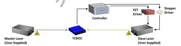
A TCBOC synchronizes the pulse trains of two ultrafast lasers at different wavelengths. Two options of the TCBOC is being offered:
